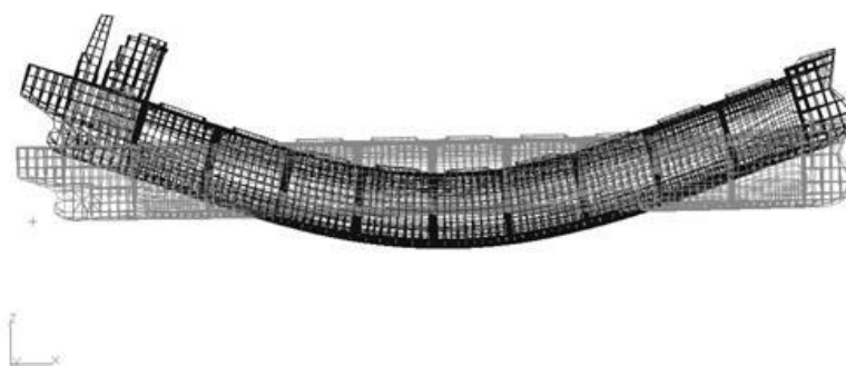
Figure 11.3.4 Mode Shape of 1st Order Vertical Vibration for a Certain Large Bulk Carrier ( f=0.462 Hz)
